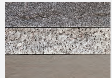
Treads Top: Blue Mist Granite Middle: Salt and Pepper Granite Bottom: Bluestone
