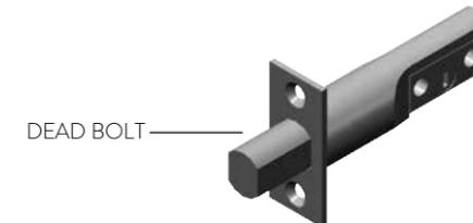
A locking mechanism that is separate from the latching mechanism in a door set. A dead bolt can be locked by a key or turn piece. Rocky Mountain Hardware can provide separate dead bolt trim that is used above a handle set or can incorporate the dead bolt and handle trim onto the same escutcheon.
