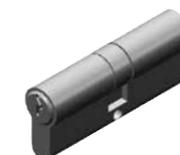
Another type of cylinder used with multi-point lock sets. These cylinders slip through the exterior escutcheon, the door and the interior escutcheon and are held in place by a set screw through the edge of the lock and vary in length for different door thicknesses.
