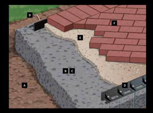
A. Compacted Sub-BaseB. 4" - 6" Compacted Aggregate (for Pedestrian Traffic)
