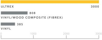
Elexural Modulus (KSI) - ASTM D790
