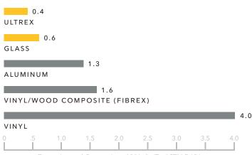
Expansion and Contraction x10<sup>-5</sup> in/in/F - ASTM D696
