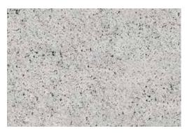
Granite, Quartz and Marble particles are embedded in the surface of the product and then revealed using additional processing methods.
